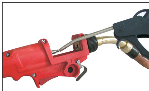
Fig. 55 Cleaning the welding torch hosepack
